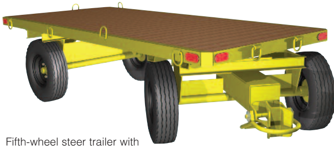
Fifth-wheel steer trailer with heavy duty automatic coupler bail rolls on solid pneumatic tires. Trailer hauls three ton loads from warehouse to air craft transport to destination.
