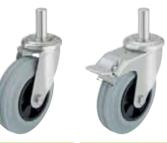
Brackets: LEXZ Series - Pressed from high-quality, chromium-nickel stainless steel (material No. 1.4301/AISI 304), swivel bracket with double ball bearing in the swivel head, plug-in stem, bolted wheel axle. All metal parts are stainless steel and brackets are vibration-ground finished.
