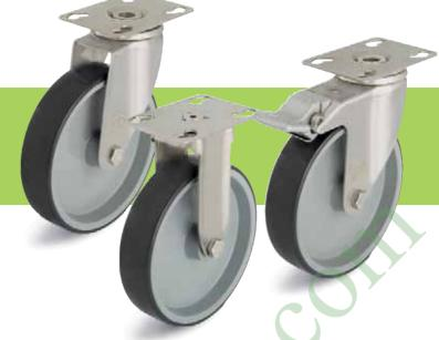
Wheels: PTH Series - Treads: Made of injection-moulded polyurethane, colour grey, non-marking, 98° shore A, abrasion-resistant, non-staining, floor-saving, low-noise operation, low rolling resistance, excellent positive and non-positive connection with the wheel centre. Wheel centres: Made of high-quality nylon, colour light grey, shock and impact-resistant, corrosion-resistant, plain bearing. Detailed description: Page 102 and 32
