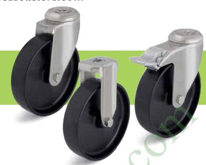
Brackets: LKRXA/BKRXA Series - Pressed from high-quality, chromium-nickel stainless steel (material No. 1.4301/AISI 304), swivel bracket with double ball bearing in the swivel head, strong central kingpin and bolted wheel axle. All metal parts are stainless steel and brackets are vibration-ground finished.
