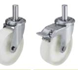
Brackets: LEXZ Series - Pressed from high-quality, chromium-nickel stainless steel (material No. 1.4301/AISI 304), swivel bracket with double ball bearing in the swivel head, plug-in stem, bolted wheel axle. All metal parts are stainless steel and brackets are vibration-ground finished.
