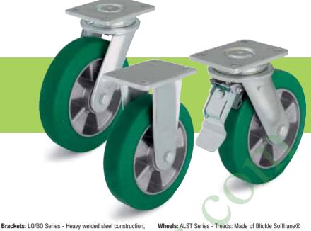
polyurethane, firmly bonded, colour green, non-marking, very high operational comfort because of particularly thick, elastic tread, 75° shore A, abrasion-resistant, high cut and tear propagation resistance, non-staining, floor-saving, low-noise operation, low rolling resistance, very good chemical connection with the wheel centre. Wheel centres: Made of aluminium die-cast. corrosion-resistant, ball bearing, colour aluminium. Detailed description: Page 210 and 44.
